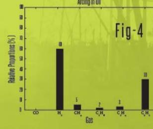
Figure-1, 2, 3 and 4 show histograms over the main decomposition products for each of the four fault types.
